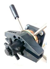
TE43 is the smallest elbow mandrel that works by replacing the standard MF3i machine sleeve with the mandrel sleeve. All the legs move the same amount when clamping so the adjustment is limited. Special liner is used for positioning the machine straight. Best results achieved when clamped very close to the end of the pipe elbow where the surface is straight.
