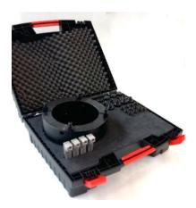
These elbow mandrels all work according to the same basic principle; Mandrel is clamped to a pipe elbow via screws on the inner diameter of the mandrel housing. Each extendable leg can be adjusted individually so centering is easily done. Legs have freely rotating heads to protect the inner surface of the pipe from damage when tightening the legs.
